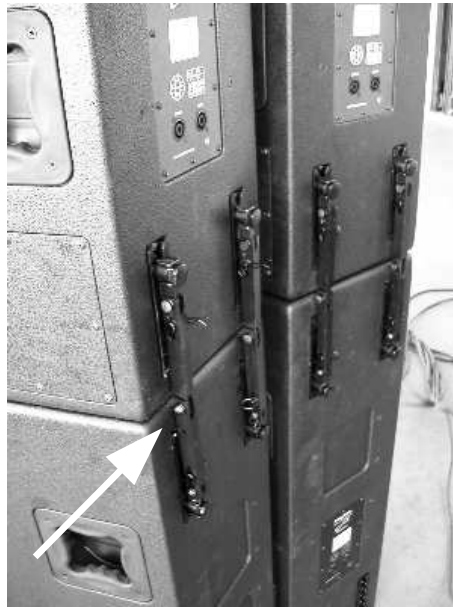
Figure 5.20: Correct positioning AC172E hinges
