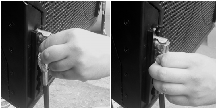
Figure 5.19: Test of the correct placing of the connection cylinders
