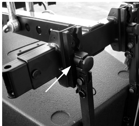
Figure 5.17: Correct position of the rear hinges in the connection of the loudspeakers to the flying bar
